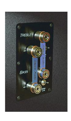
To facilitate proper set-up of your speakers in a variety of room situations, we have included several heavy duty toggle switches on the terminal plate, located on the back of the loudspeaker. All switches in the "up" position represent the "anechoic flat" position.
